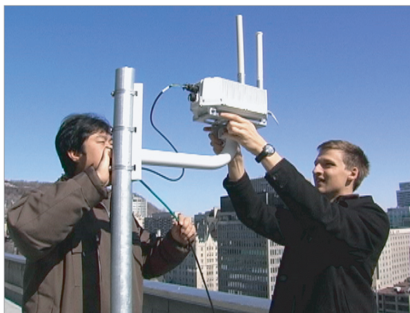
Outdoor wireless mesh access point located on the rooftop of a downtown university building.
